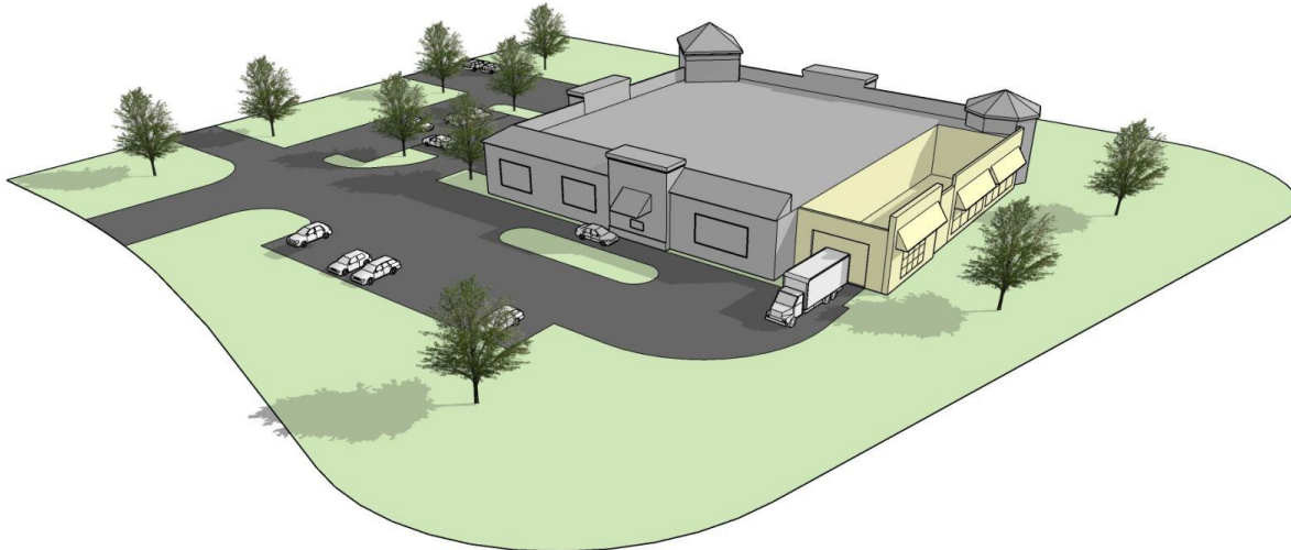
Figure 3.03.04 Illustrative Example of Enclosed Loading
