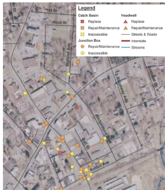
2009 Condition Assessment – Structures
